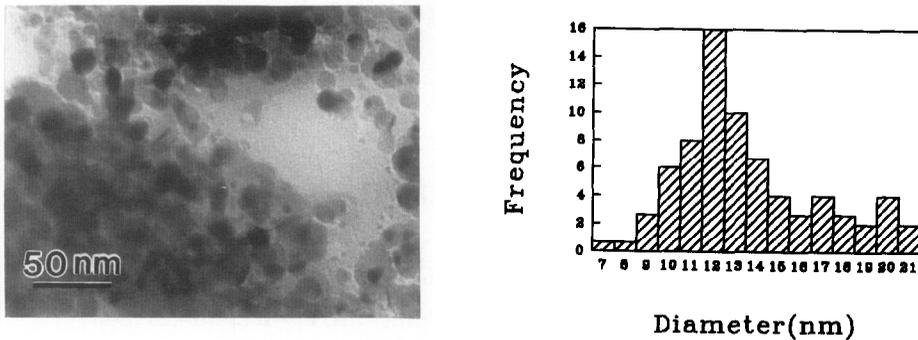
Figure 1. TEM micrograph and particle size distribution for nanocrystalline Ni with average particle size around 12 nm.
