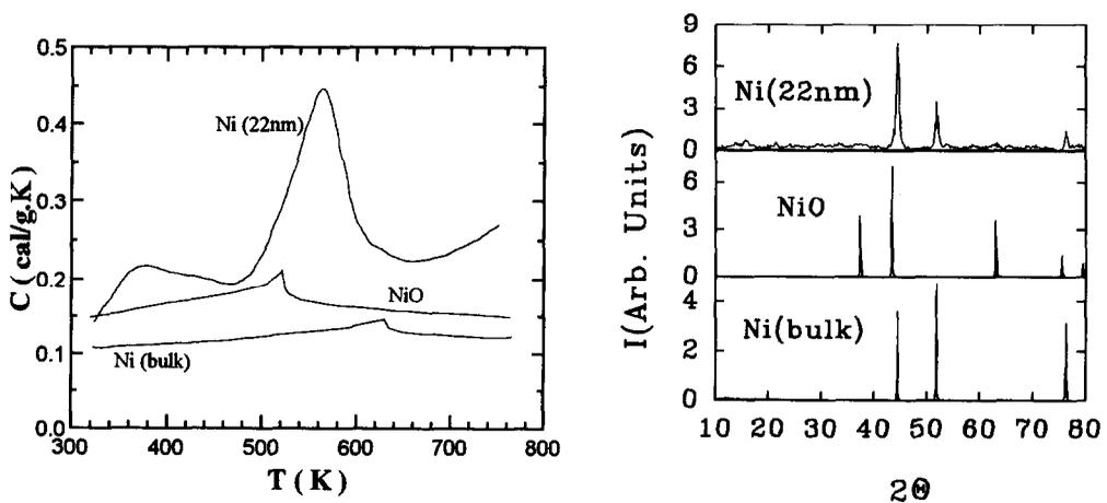
Figure 2. Specific heat of bulk Ni, nanocrystalline Ni (22 nm) and NiO between 300 and 800 K.
