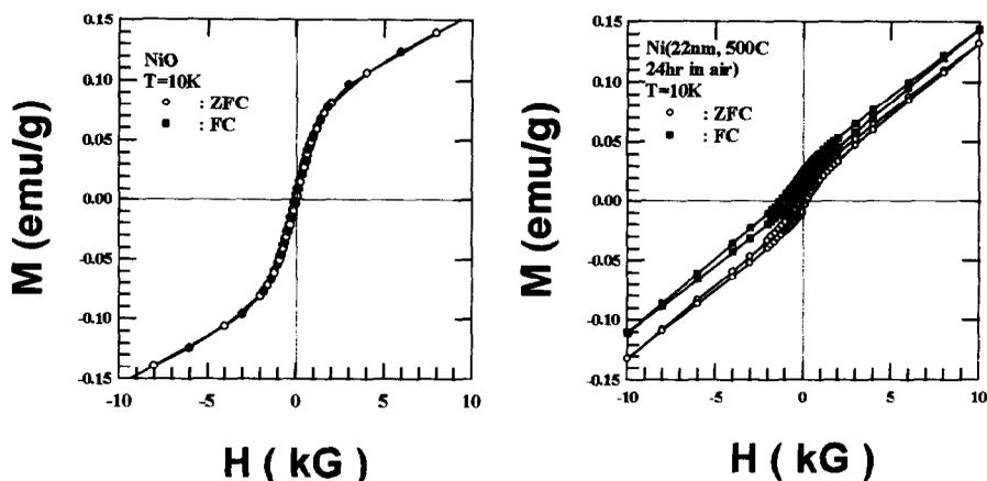
Figure 5. FC & ZFC curves of  $M$  vs  $H$  at  $T=10$  K for NiO and Ni (22nm) annealed at 500 C in air for 24 hrs.
