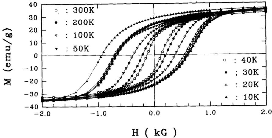
Figure 3. Field (8 kG) cooled M vs H curve for Ni particles with 22 nm at different temperatures.
